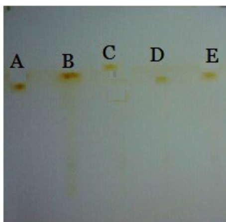
Figure 2: TLC sheet showing good retardation of crude sample with ethyl acetate and benzene (2:8).
