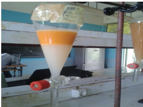
Fig.8: Glycerol separation using water
