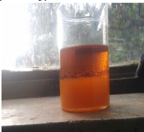
Fig.5: Transestrification reaction and biodiesel layer
